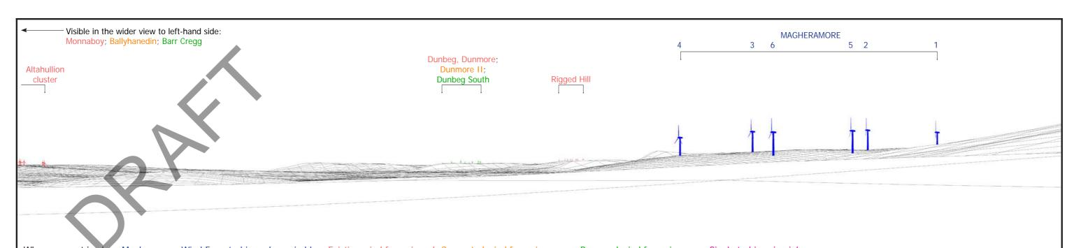
Where present in view: Magheramore Wind Farm turbines shown in blue; Existing wind farms in red; Consented wind farms in orange; Proposed wind farms in green; Single turbines in pink Turbine dimensions shown for the Development: max. tip height above ground level 149.9 m; hub height 94 m; rotor diameter 112 m
